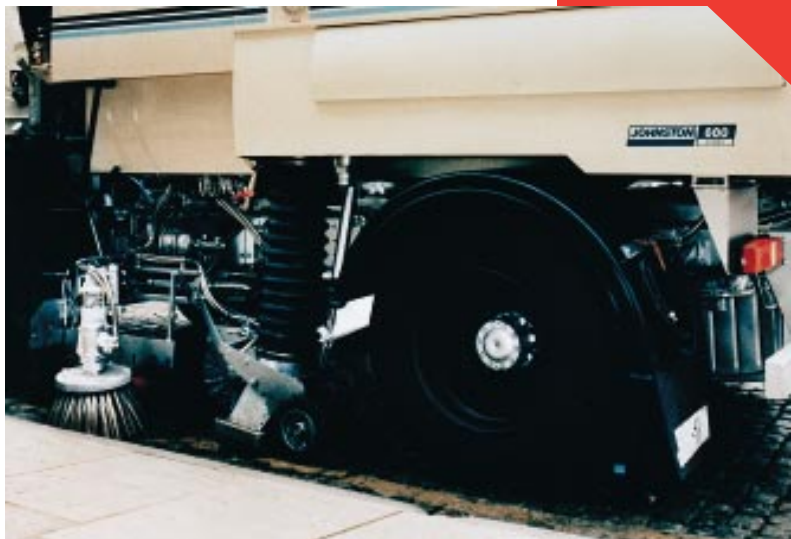
A Linaplus OZ flexible hose fitted to a road cleaning vehicle
